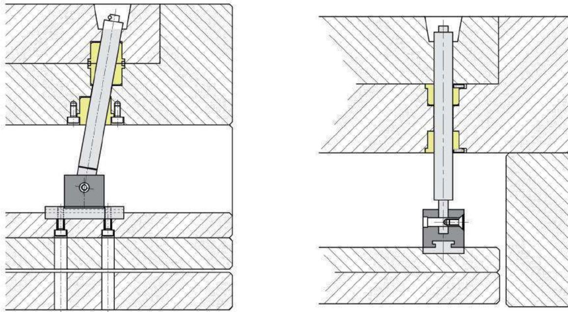
Fitting example of box type angular lifters with guide bush
